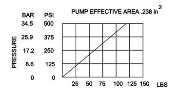
FORCE ABOVE CURVE IS WITH HYDRAULIC OIL 150 SSU AT 100°F.
