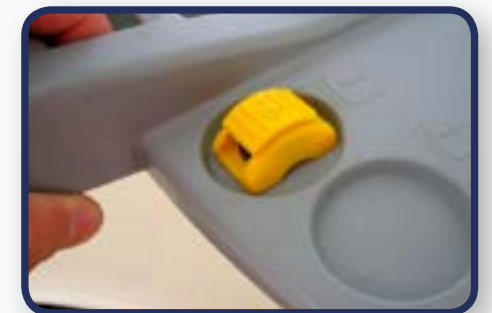
STACKERS PROPORTIONAL ROLLER FOR LIFT & LOWER CONTROL
