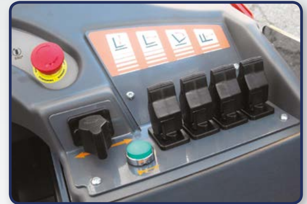
IN CABIN CONTROL FINGER-TIP PROPORTIONAL CONTROL LEVERS
