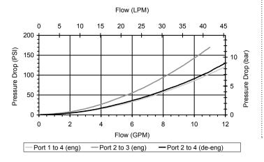
For higher pressures see HG-S4C. Operational shift limit, 8 GPM (30 LPM). For shift performance consult chart.
